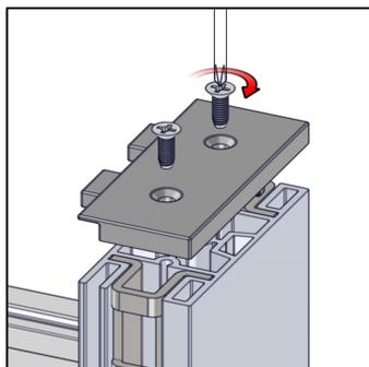
LOOSEN END CAP TO ATTACH
